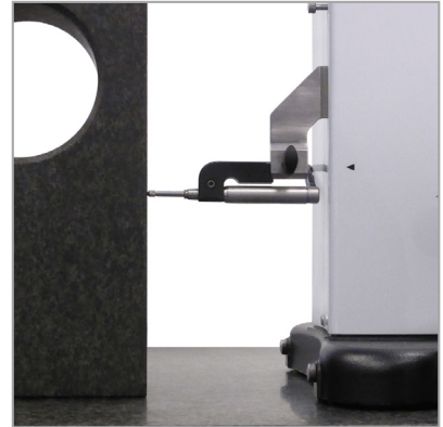
Perpendicularity measurements with electronic probe (TA-IH-126, TA-MS-101)
