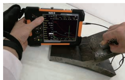
● Angle weld testing
