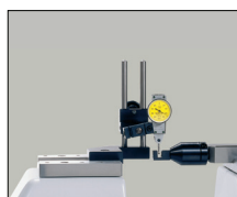
Checking of test indicators
