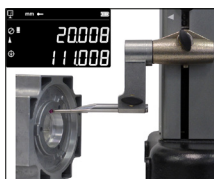
Simultaneous display of diameter and centerline
