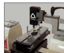
Calibration of small ring gauges
