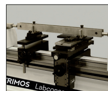
Comparative checking of gauge blocks > 250 mm
