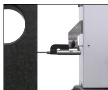
Perpendicularity measurements with electronic probe
