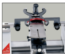
Checking of snap gauges
