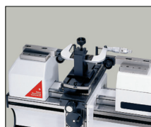
Calibration of external micrometers
