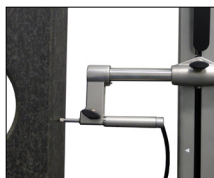
Squareness measurements with electronic probe
