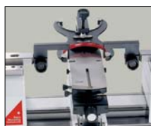
Checking of snap gauges
