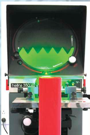
Measurement of Angle on Profile Projector
