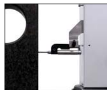
Perpendicularity measurements with electronic probe
