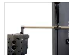
Standard measuring inserts up to 400 mm, with excellent repeatability
