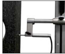
Squareness measurements with electronic probe
