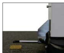
Height measurements on watch movement plate
