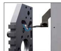
Minimum position measurement thanks to the contour tracking in motorized mode
