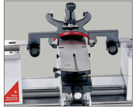
Checking of snap gauges (TA-SU-313/TEL14N)
