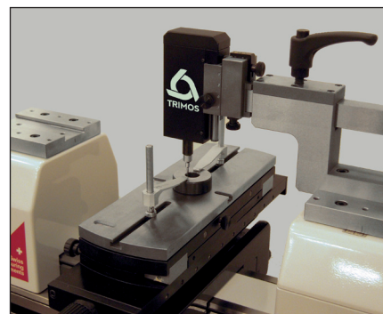
Calibration of small ring gauges (TA-SU-313/LABC-70/TA-SU-354)
