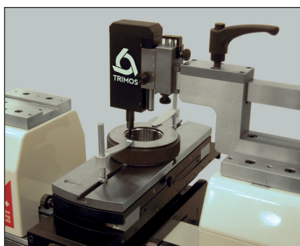
Calibration of thread ring gauges (TA-SU-313/LABC-70/TA-SU-354)
