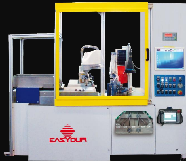
FLEXI ROTARY ROBOT AUTOMATIC FEEDING + COMPRESSION + VISION + SORTING
