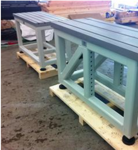
T-slot table with custom support frame
