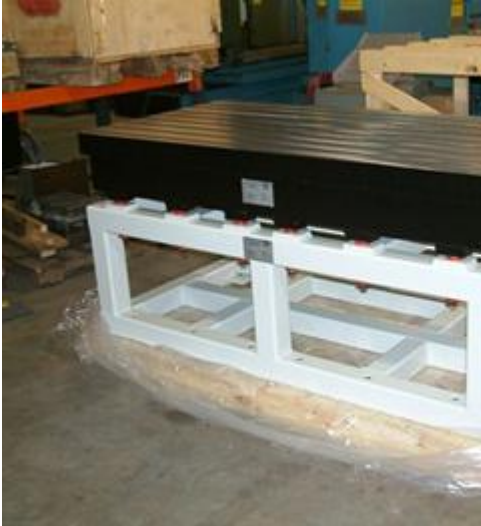
Steel T-slot Table on a heavy support frame with a first natural frequency >100 Hz size approx. 1800 x 900 x 800 mm
