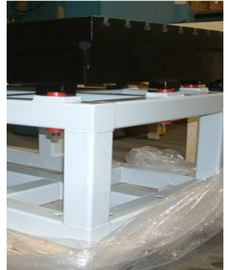
Isolation pads for vibration decoupling between table plate and frame
