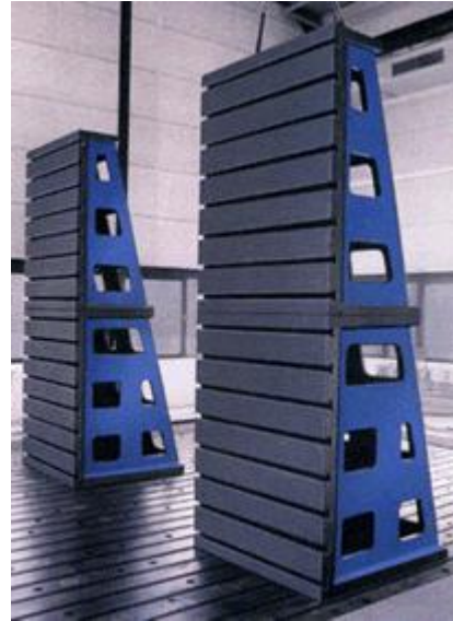
A matched pair of angle plates each in two-piece construction, height 4000 mm, mounted on an isolated foundation floor plate for highly dynamic testing
