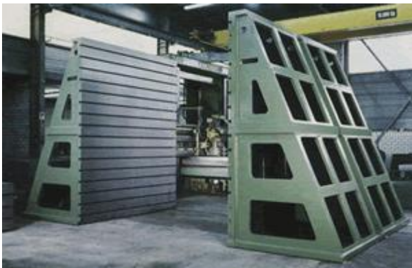
Angle plate for heavy duty cutting work. Plate surface 3500 x 2500 mm
