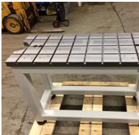
T-slot table with custom cut-outs for accessories
