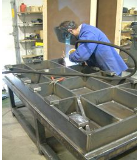
View of the table bottom with welded rib design
