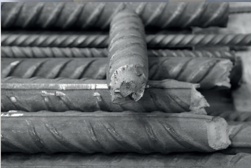
Result of tensile tests on rebars
